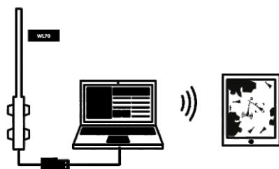
With the WL70 you can utilise windows connection sharing on your laptop or PC which will act as a wifi router allowing other mobile users with iPads and tablets to share the connection. It can also be used with the iKConnect router (with USB connection)
