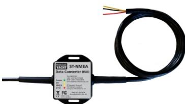
The SeaTalk\* to NMEA (ISO) gateway is a small but powerful interface that provides bi-directional conversion between a SeaTalk network and an NMEA 0183 network or device. Taking its power from the SeaTalk network, the ST-NMEA gateway features a protected SeaTalk 1 interface, an opto-isolated NMEA 0183 input and differential NMEA 0183 output that allows key navigational data to be reliably shared between the SeaTalk and NMEA 0183 networks. USB version also available.
